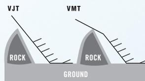
The VJT sidewalls are designed with more rigidity and are shaped for more ground clearance at the edge to minimize cutting damage from sharp objects.
