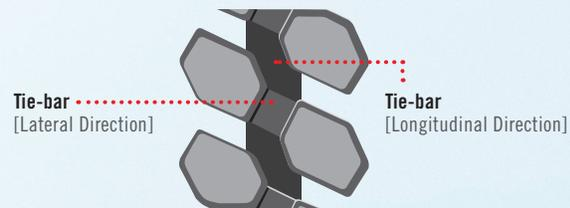
The VJT's double-reinforcing tie bars increases center block strength for enhanced wear resistance. The longitudinal and latitudinal tie bars minimize the center blocks elongation and deformation upon surface contact. This reduction in friction between the center blocks and the ground minimizes irregular block wear and extends tire life.
